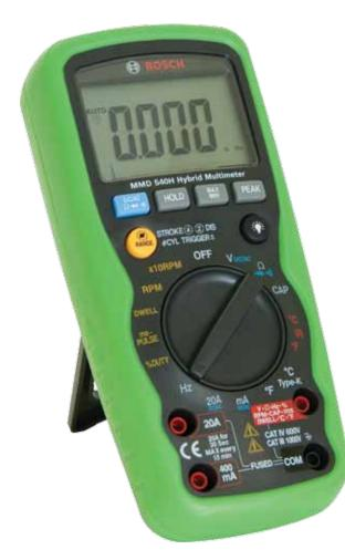
The Bosch MMD 540H Hybrid Multimeter is a CAT safety rated, auto ranging digital multimeter designed for use in diagnostics of electronic circuits. Whatever your shop services: automotive, fleet, motorcycle, marine or small engine, the MMD 540H has the capability to keep up with your business.
