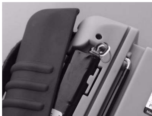
FIGURE 1-7. Battery in Its Compartment behind the Rubber Grip
